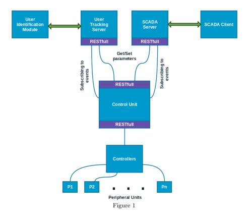
best suite the identified user. The control unit is directly connected to the controllers that are responsible for controlling individual peripherals. The actual peripherals and their controllers are independent of the system. Communication between entities of the system is made by utilizing TCP/IP protocol with Secure Sockets Layer (SSL) encryption. The topology of the system is shown in Figure 1.
