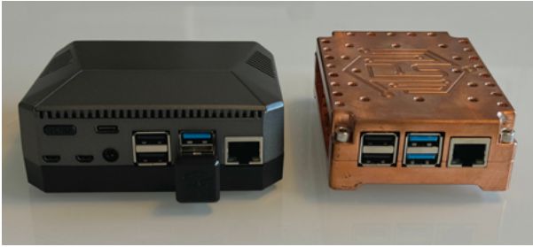
Figure 7.2 Raspberry Pi 4 in DiSalvo copper enclosure (right) and in Argon ONE M.2 enclosure (left)
