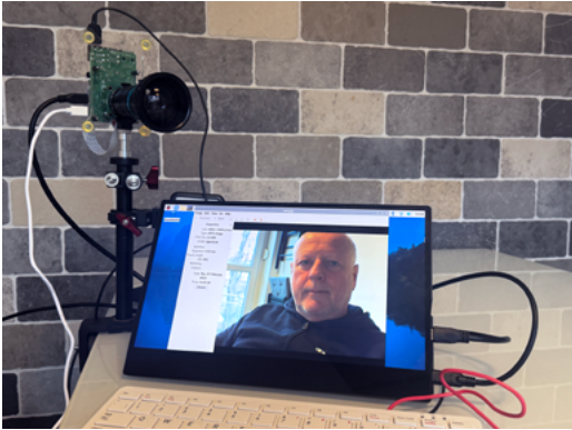
Figure 4-5 Capturing images with Raspberry Pi 4 and a HQ camera
