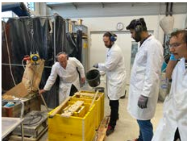
Ulivanje recikliranega betona v modele Pouring of recycled concrete into the molds
